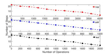
Figure 12: The depth of SPOILER leakage with respect to different instructions and execution units.
